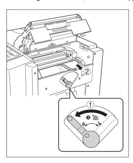
Insert the leading edge of the Master Roll into its entrance under the Master Guide Flap.
