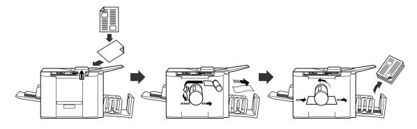
A placed original is scanned by the scanner, and a generated master is rolled around the Print Drum (Cylinder). After a while, sample copy is performed. After checking the print result, enter the number of pages to be printed and start printing.
