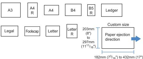
• Paper weight:  $46g/m^2$  -  $210g/m^2$  (12-lb bond to 56-lb bond) ( $60g/m^2$  to  $220g/m^2$  [16-lb bond to 58.7-lb bond] for cover sheet)
