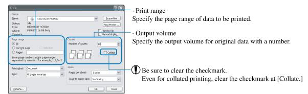
If you click the [Properties] button, you can set the various conditions on the printer driver screen. The settings of [Original image] on the [Main setting] tab and [Paper type] on the [Main setting] tab affect seriously the print quality. When using conditions other than the default settings, click the [Properties] button and adjust the settings.
