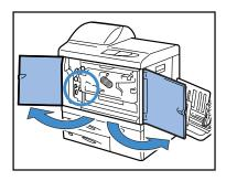
2 Turn Dial A and remove the paper from the Transfer Roller side.
