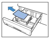
**3** If the paper cannot be removed, open the Transfer section door at the left side of the Feed Tray and remove the paper.
