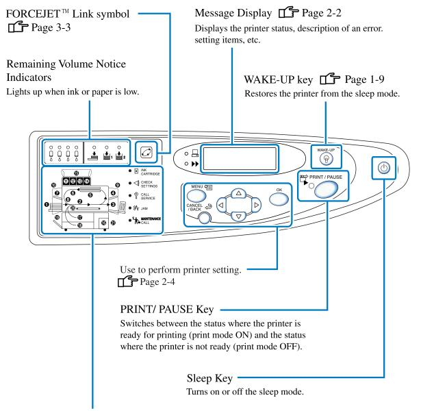
Indicates the description and location of an error when a paper jam occurs inside or a cover is not securely closed.
