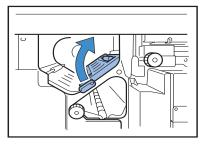
3 While turning Dial B in the direction indicated by the arrow, remove the paper.
