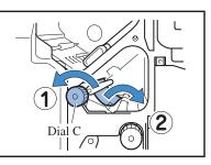
6 Return the tab at the left of the Reversing Path Cover to its original position.
