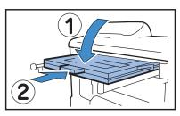
7 Return the tab at the left of the Reversing Path Cover to its original position.
