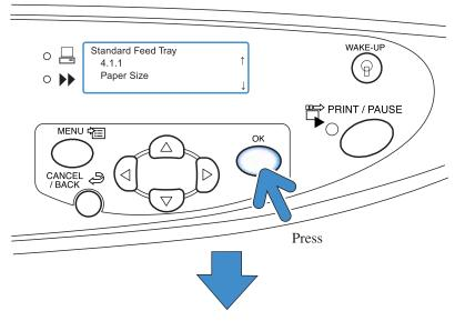
Menu setting can be performed. Press the  $\triangle$  or  $\bigtriangledown$  key to select the desired item and press the OK Key.
