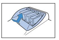
2 While lifting the lnk Cartridge to be replaced, pull it toward the front side and remove it.
