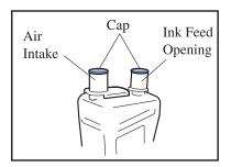
5 Hold the surface of the lnk Cartridge with the ▲ mark up and insert the cartridge until it stops.
