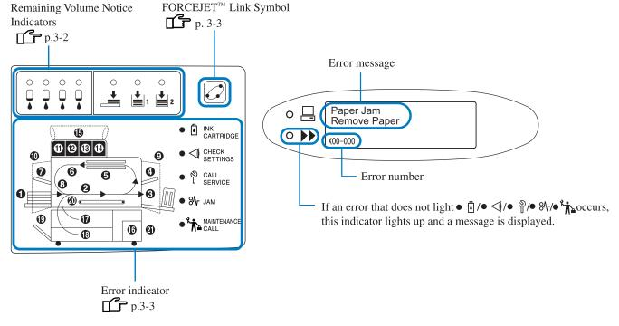
If [21] in the panel is lit, an error occurs in the optional HC Finisher. For details, refer to "HC Finisher Maintenance Guide."
