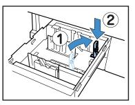
4 Load paper by positioning the centre of the paper to the centre mark (▼) inside the Paper Feed Tray.
