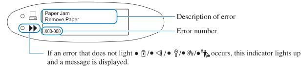
When an error occurs, an error number and its description are displayed in the Message Display. For error numbers, refer to "Chapter 3 Troubleshooting" \$\varphi\$ p.3-1.
