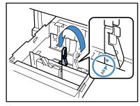
When loading A3/Ledger size paper, do not use the Paper Top Guide. Remove the Paper Top Guide and insert it into the holder in the Paper Feed Tray.
