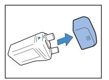
4 Remove the two caps from the ink feed opening and the air intake.
