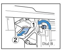
4 If the paper cannot be removed, open the Left Transfer Path Cover and remove the paper.
