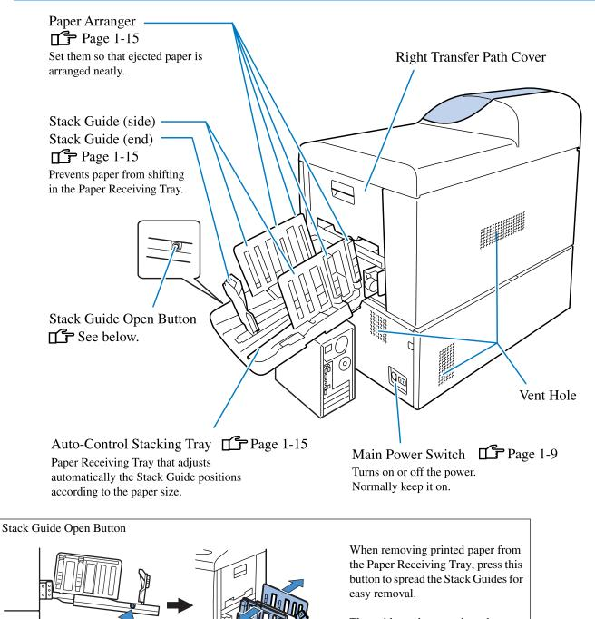
The guides to be spread can be set. For details, refer to "4.8.4 Shifting Guide" of the menu setting . \* p.2-27
