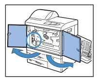
2 Turn the Transfer Lock Lever to the left and turn down the tab to the right.
